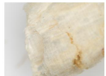
Figure 5. Kenaf particles have a highly textured surface to support biofilm growth.
