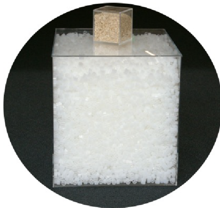
Kenaf biomedium (top) and the equivalent surface area of plastic media
