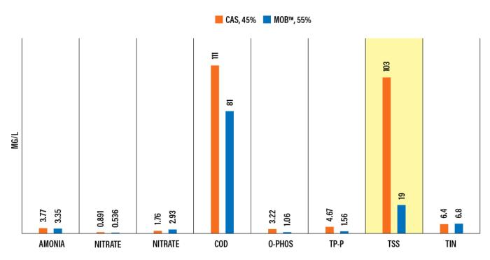
The MOB™ Process had 1/5 of the TSS in the effluent compared to the CAS reactor.
