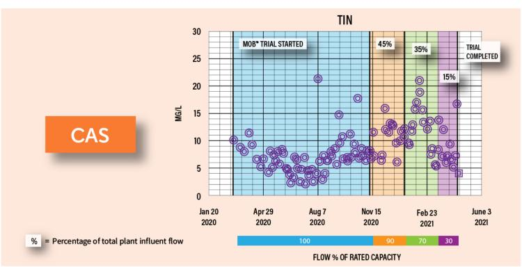
CONTROL & DECREASE OF EFFLUENT TOTAL NITROGEN AT MOB™ PROCESS ELEVATED FLOW
