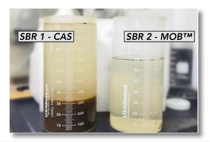
CAS effluent had a settled sludge volume of approximately 300 mL/L, while MOB™ effluent had no observable sludge volume after the same settling time during high flow event ( > 10x design).
